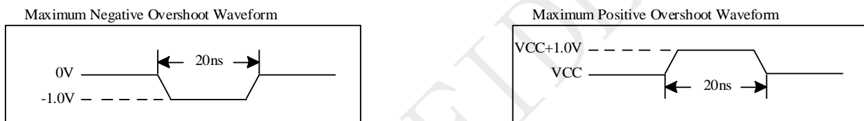
Figure 5-1 Maximum Overshoot Waveform
