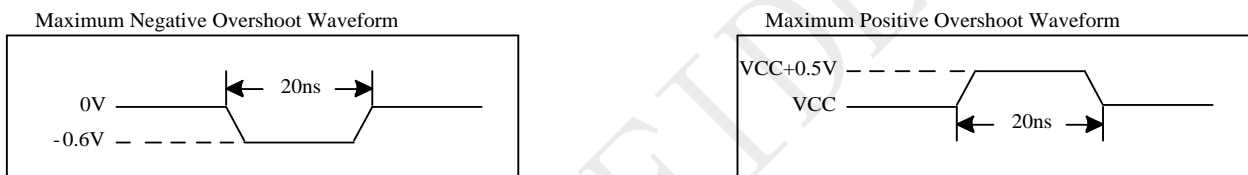
Figure 5-1 Maximum Overshoot Waveform
