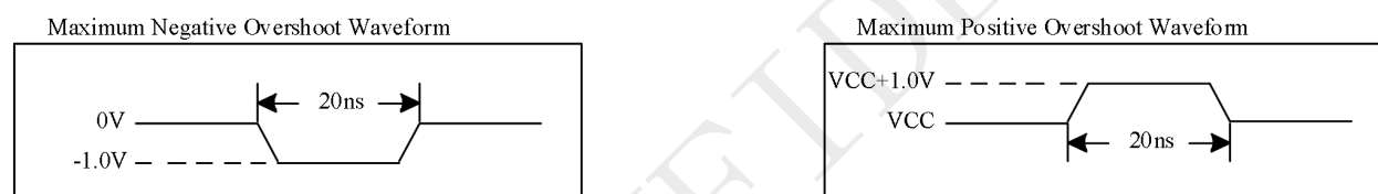
Figure 5-1 Maximum Overshoot Waveform
